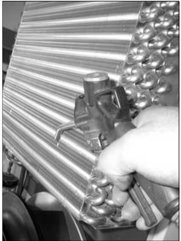
Fig. 55: Clean out the heat exchanger coil and compressor chamber using compressed air (1)
