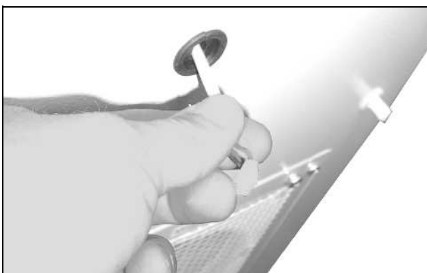
Fig. 65: Push back the display cable and press it through the cable gland (1)
