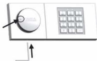
Fig. 5.1: Note the position of the rotary handle (marking). Insert the Allen wrench into the small hole on the bottom side and press it in to the stop.
