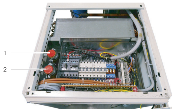
Fig. 24: Connection points on the top of the unit
