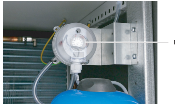
Fig. 64: Adjustment screw at the differential pressure sensor
