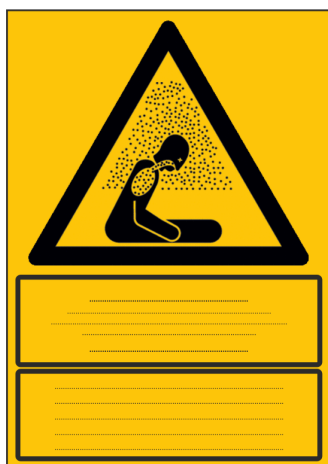
Fig. 2: Marking of the extinguishing zone (example)
