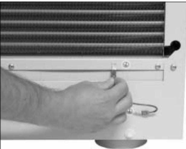
Fig. 35: Disconnect the earthing cable
