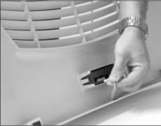
Fig. 34: Disconnect the connector from the display
