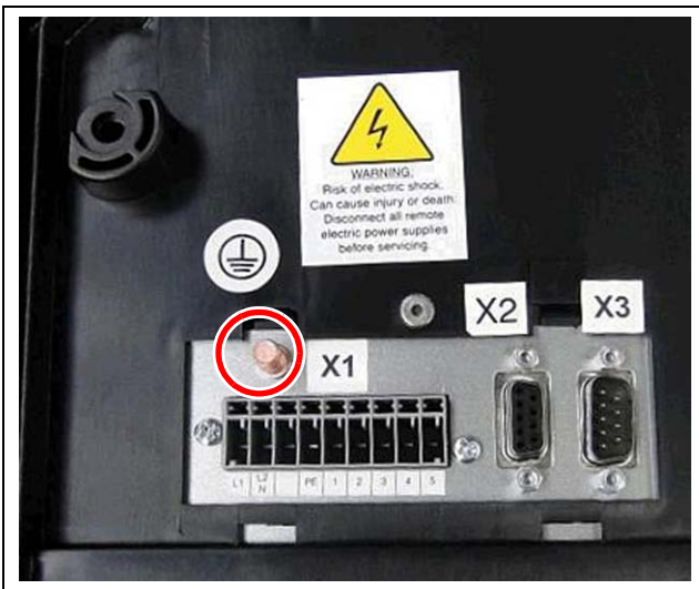
Fig. 13: Connection point, potential equalisation
