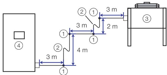
Fig. 21: Simplified representation of connection lines
