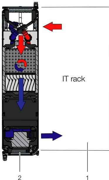
Fig. 46: "Front to back" cooling principle with bayed LCP Rack
