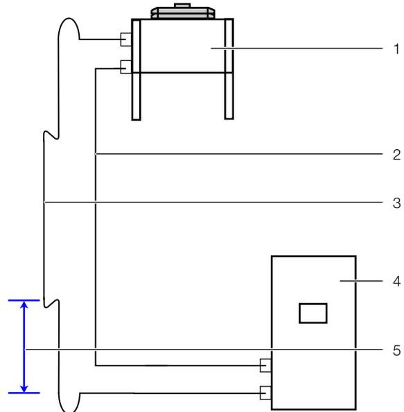
Fig. 20: Oil elevation arc
