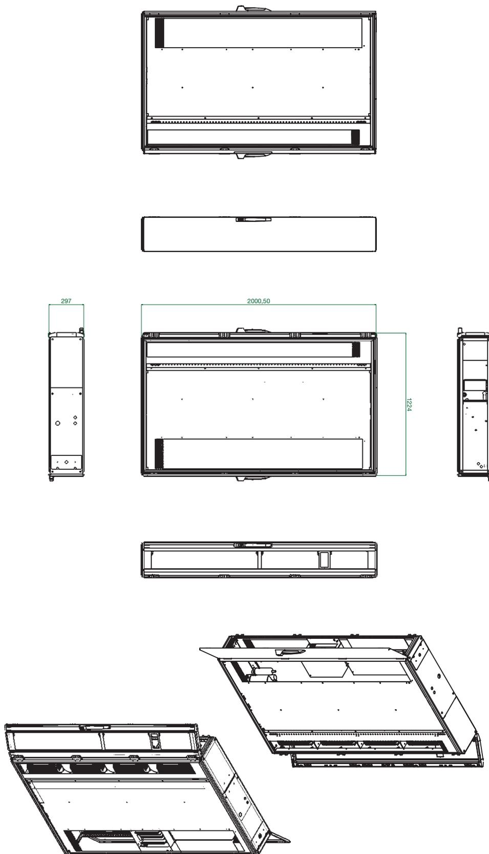
Fig. 42: Overview drawing of the LCP DX (depth 1200 mm)
