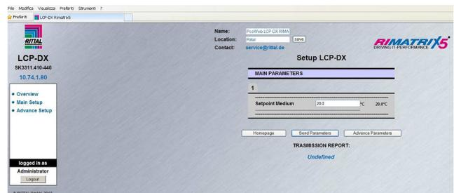
Fig. 27: Setting the server air injection temperature
