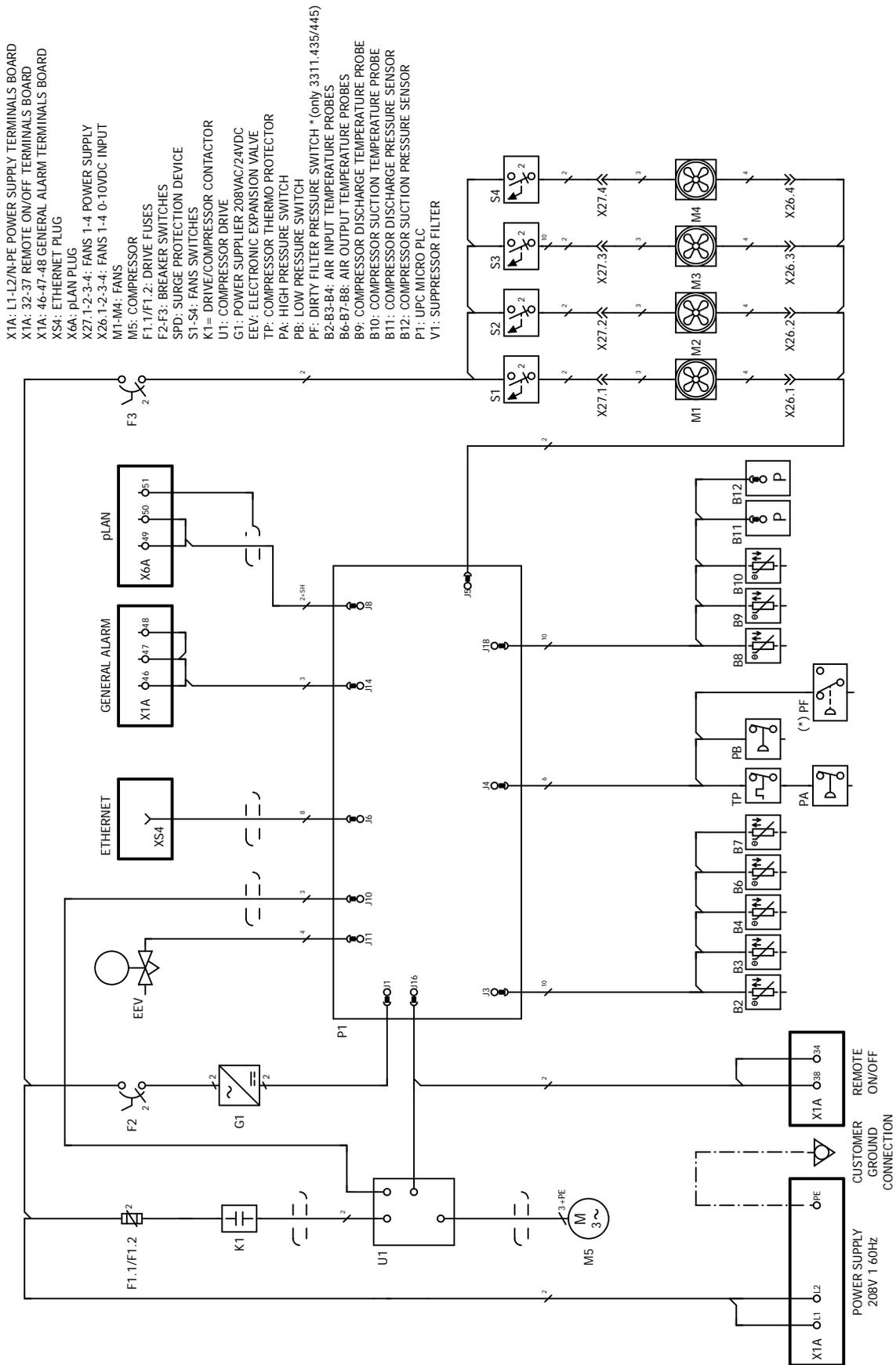
Fig. 44: Circuit diagram of the LCP DX
