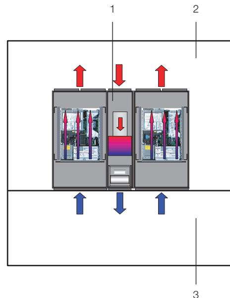
Fig. 14: Installation room with cold aisle containment
